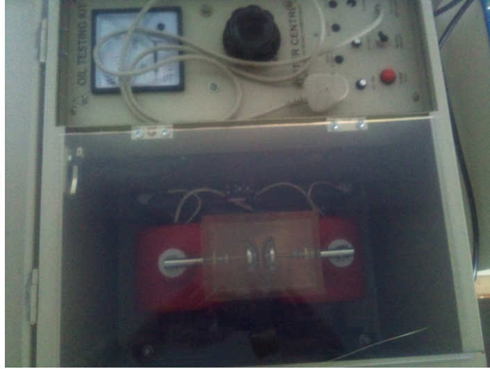
Fig 6 Arrangement of Transformer Oil Testing Kit
