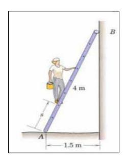
**8.** A 4 m ladder weighing 200 N is placed against a vertical wall as shown in Fig. 4.2 as a man weighing 800 N, reaches a point 2.7 m from *A*, the ladder is about to slip. Assuming that the Coefficient of friction between the ladder and the wall is 0.2, determine the coefficient of friction between the ladder and the floor.
