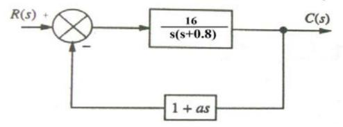
(5) Determine the value of 'K' and 'a' such that the system has a damping ratio of 0.7 and an undamped natural frequency of 4 rad/sec for the system shown below
