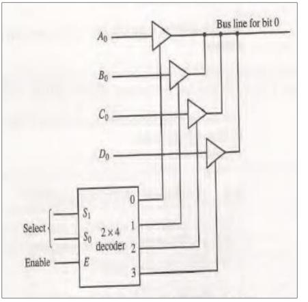
A bus system can also be constructed with three-state gates. A three-state gate is a digital circuit that exhibits three states. Two of the states are signals equivalent to logic 1 and 0 as in a conventional gate. The third state is a highimpedance state. The highimpedance state behaves like an open circuit, which means the that output **1**S disconnected and does not have a logic significance.
