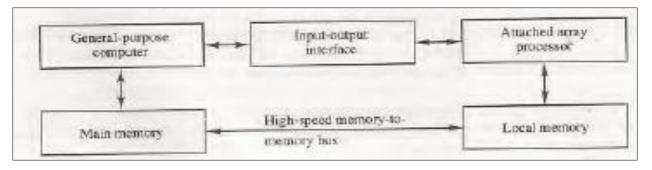
Attached array processor with host computer.
