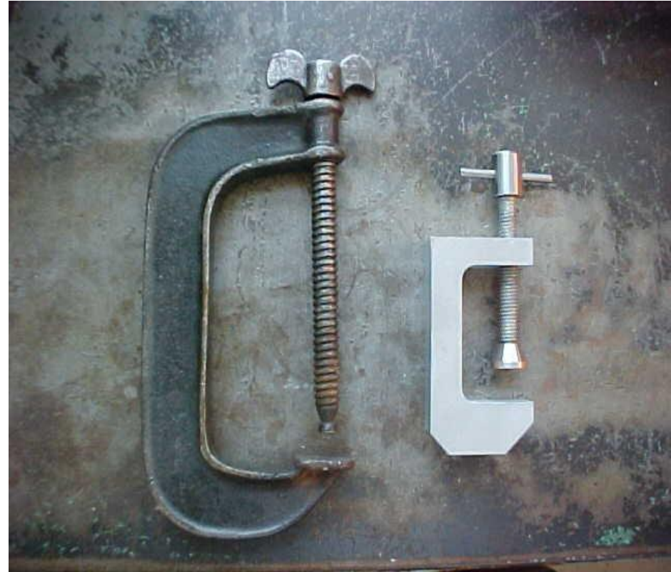
C-clamps formed by casting (left) and machining (right)
