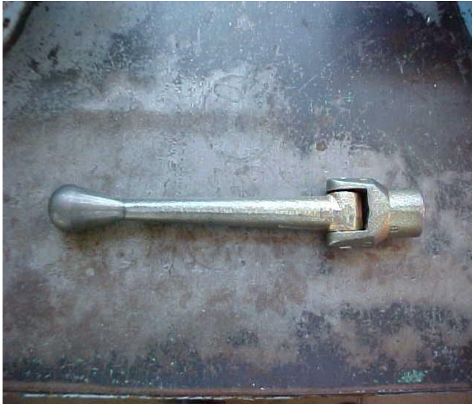
Crank handle formed by casting; some areas were machined and assembled after casting
