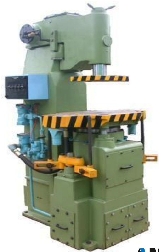
Fig. 2.7.3 : Schematic diagram for air operated jolt squeeze machine
