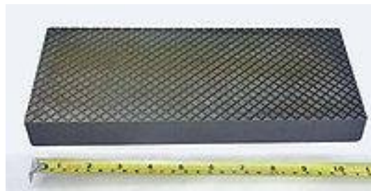
Fig 12.6 Small lapping plate made of cast iron
